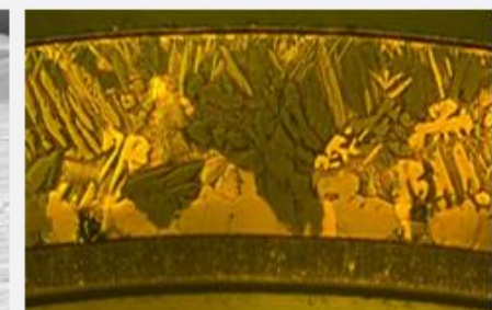
After HT oxidation test at 1200°C for 2000s
